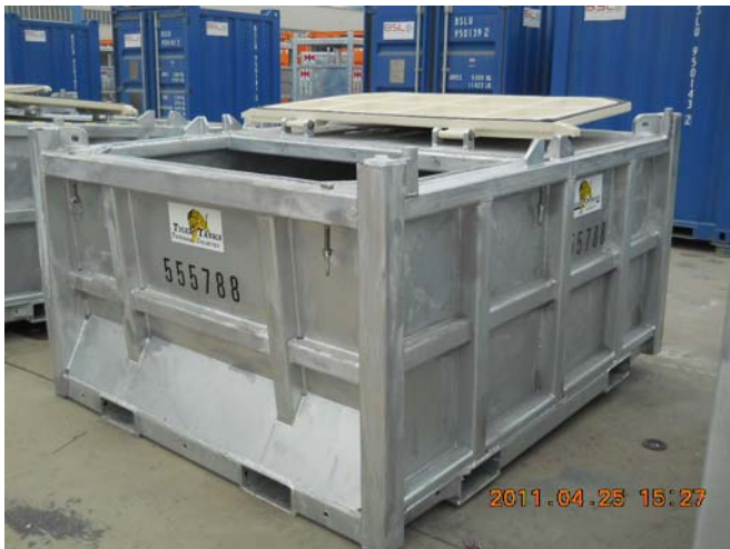
Drilling cutting box with galvanized surface
