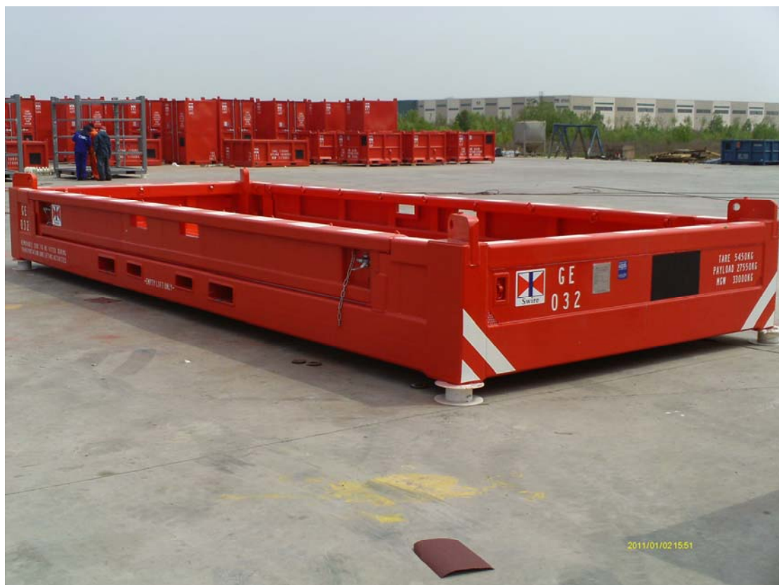
7.3M HEAVY LIFT HALF HEIGHT OPENTOP OFFSHORE CONTAINER
