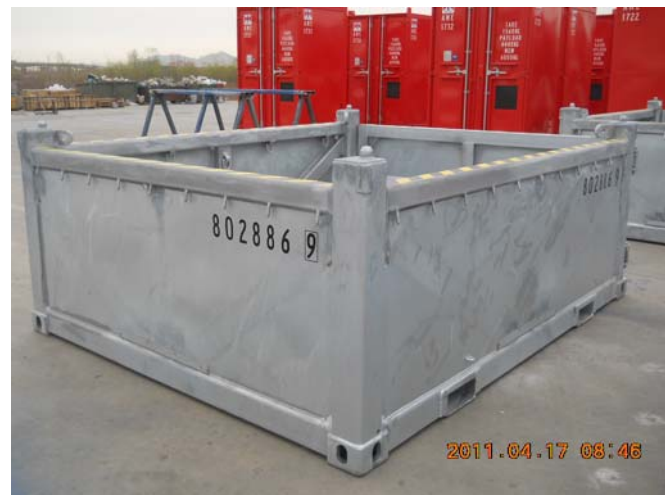
10' half height container with galvanized surface
