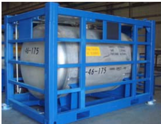
4600 Liters Horizontal offshore tank (IMDG T7)
